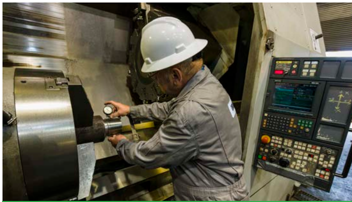
Tubular connection repair services include providing API stress-relief groove pins and bore back boxes, cold rolling thread roots, and phosphate coating to help prevent galling.
