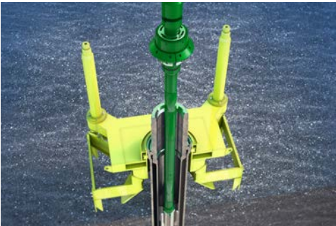
The casing is severed mechanically and the wellhead spear remains engaged for a simultaneous retrieval of the casing section and wellhead.
