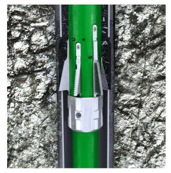
A section milling application with WavEdge\* technology was used successfully in a remedial application to optimize production in an aged well in the Gulf of Guinea. The success of this application and the value generated was recognized by the customer.
