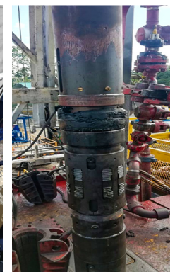
Figure 4: Successful recovery of lower Quantum Packer.
