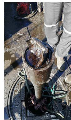
Figure 3: Broken 3½ in. production tubing pieces inside the upper Quantum packer.
