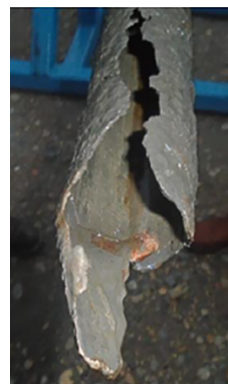
Figure 1: Heavily corroded 3½ in. production tubing.
