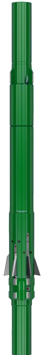
*Three cutter arms automatically expand into the milling position when the K-Master mill cutout arms are fully open.*
