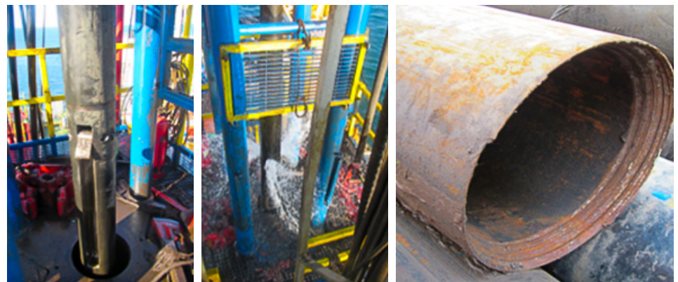
WIS hydraulic casing cutter tandem with 7 inch OD mud motor.
