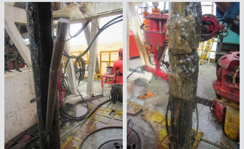
Figure 4: Recovered wireline tools previously lost in hole without any records.
