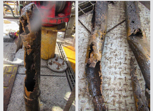
Figure 1: Recovered corroded tubing.
