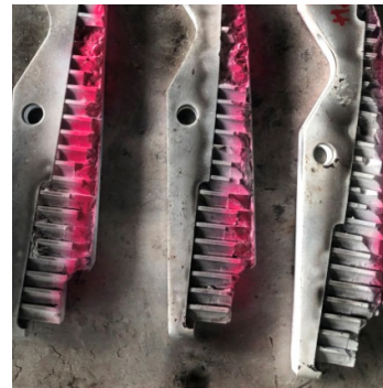
ProMILL Duo knives with only 20% wear after milling the required interval in a single trip
