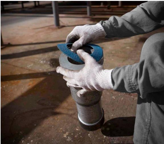
The refacing tool is rotated by a heavy-duty electric sander and the pressure is applied by the operator along the axis of the threaded connection (Fig. 100). The drive tube is made from aluminum to reduce the weight of the assembly.
