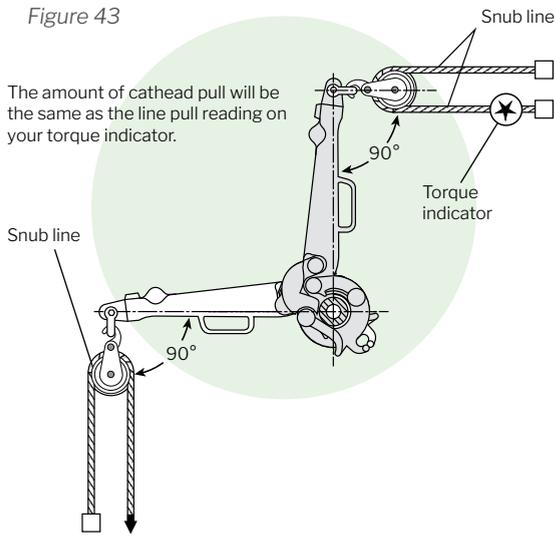
The amount of cathead pull will be the same as the line pull reading on your torque indicator.
