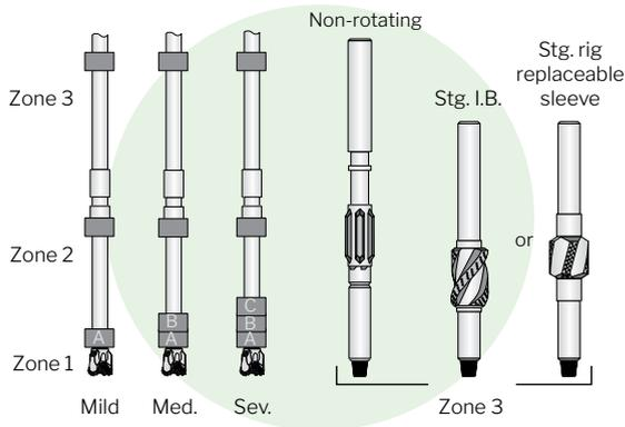
Any stabilizers run above Zone 3 are used only to prevent the drill collars from buckling or becoming wall stuck, and in most cases, will have very little effect on directing the bit.
