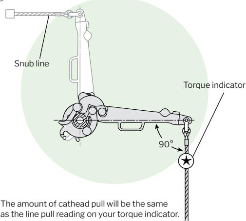
The amount of cathead pull will be the same as the line pull reading on your torque indicator.
