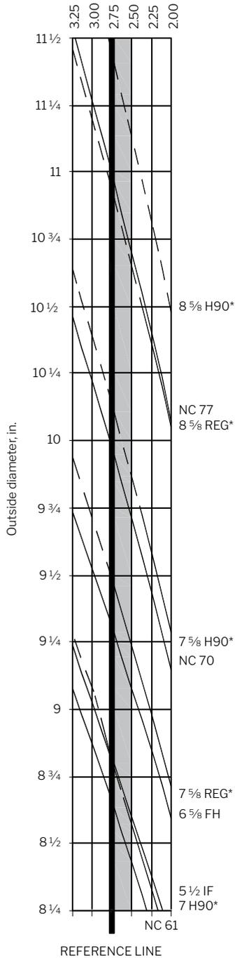
† On ODs where these connections are noted by a dotted line, they must be machined with a low torque face for proper makeup. (See page 69 for explanation of low torque face.)
