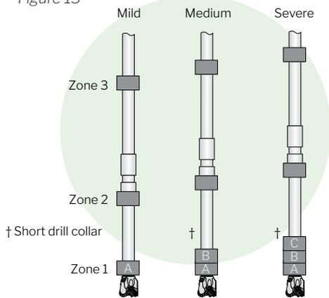
† The short drill collar length is determined by the hole size.
