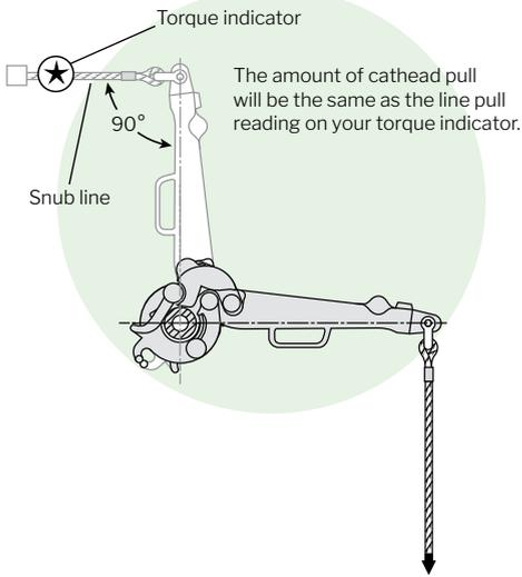
The amount of cathead pull will be the same as the line pull reading on your torque indicator.
