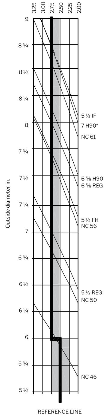
† On ODs where these connections are noted by a dotted line, they must be machined with a low torque face for proper makeup. (See page 69 for explanation of low torque face.)
