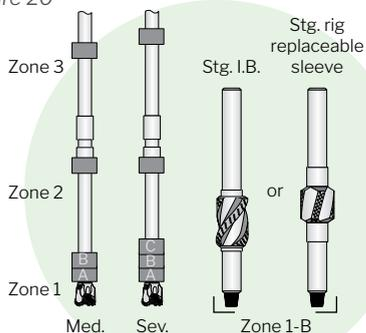
**Note:** The same tools would be used in Zone 1-C for severe crooked hole country.
