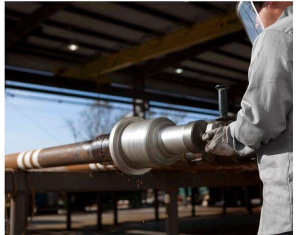
Extreme care should be taken in removing only the minimum amount of material required. When making field repairs, operators of the tool should be skilled and understand service conditions of the product to assure the proper application of the refacing tool. It is a good practice not to remove more than  $\frac{1}{32}$  in. (0.8 mm) from a box or pin shoulder at any refacing and not more than  $\frac{1}{16}$  in. (1.6 mm) cumulatively (see API Recommended Practice RP 7G, current edition).
