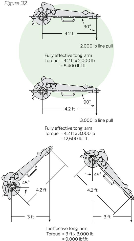
3. A line pull measuring device must be used in making up drill collars. It is important that line pull be measured when the line is at right angles (90 degrees) to the tong handle.
