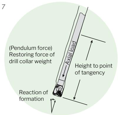
Woods and Lubinski work made it possible to utilize gravity as a means of controlling change in the hole angle. Special tables were prepared to show the necessary weight for the bit to maintain a certain hole angle. These tables also show the proper placement of a stabilizer to give the maximum pendulum force and the maximum weight for the bit. The effects of using larger drill collars can also be determined.
