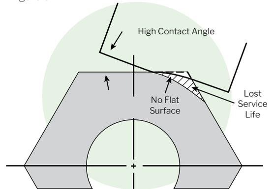
**Worn kelly with worn drive assembly.** The drive edge is a curvature with a high contact angle.
