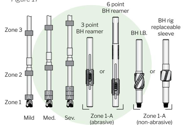
**Note:** Use a reamer if the bit gauge is a problem. Use a 6 point in extremely hard and abrasive formations.
