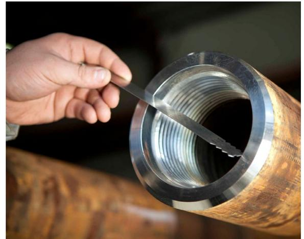
Pin base diameters can vary widely on the same size joints, but no inaccuracies will be experienced if the nearest size is read and coupled with the correct number of threads per inch. As an example, 3½ FH, 3½ IF and 3½ H-90 have nearly the same pin base diameter, but can be easily distinguished by the number of threads per inch.
