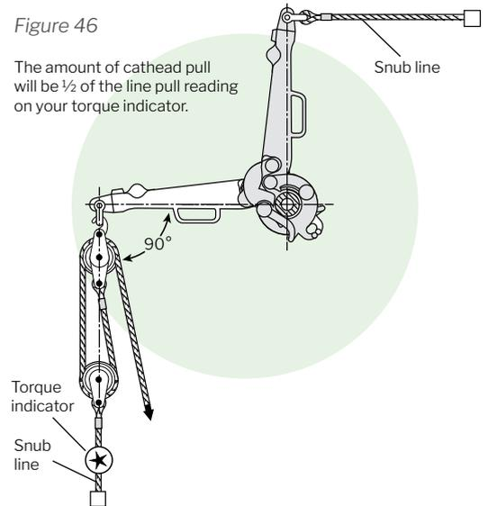
The amount of cathead pull will be  $\frac{1}{2}$  of the line pull reading on your torque indicator.
