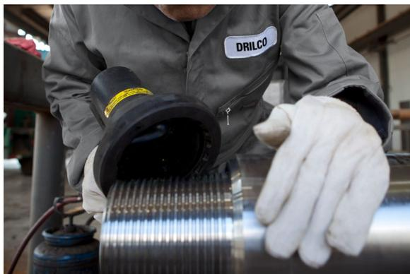
If a crack indication is found, the inspector polishes it with a soft fibrous wheel to verify the presence of a fatigue crack (Fig. 93). The inspector then re-cleans, re-magnetizes and re-sprays the connection with the fluorescent magnetic particles and re-inspects with the UV light to verify that the indication is a crack.
