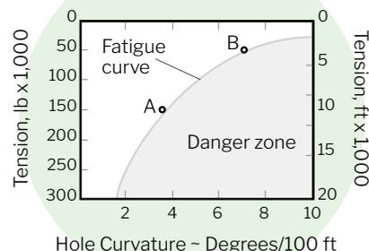
If the stress endurance limit of the drillpipe is exceeded due to rotation through a dogleg, an expensive fishing job or a junked hole could develop.
