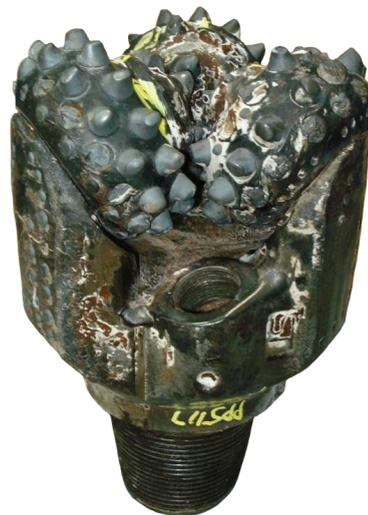
Figure 28 shows a medium formation bit that has suffered gauge wear and gauge rounding due to angular misalignment.
