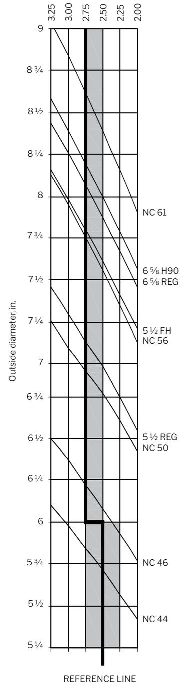
† On ODs where these connections are noted by a dotted line, they must be machined with a low torque face for proper makeup. (See page 69 for explanation of low torque face.)
