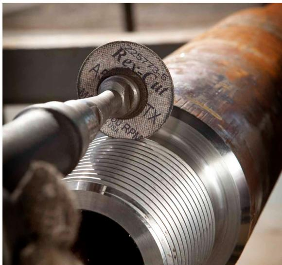
As part of the inspection record, the drill collar serial number, tally length, OD and ID are noted. Also, connection size and type, field repairs made, and number of connections inspected are recorded. Joints requiring shop repairs are clearly marked to
