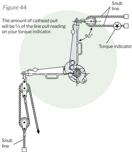
The amount of cathead pull will be  $\frac{2}{3}$  of the line pull reading on your torque indicator.
