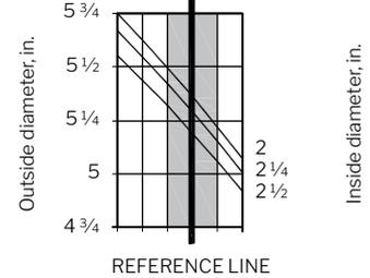
**Caution:** The use of the 90° thread form on drill collar sizes less than 7½-in. OD may result in hoop stresses high enough to cause swelled boxes. For this reason the API 60° thread form is preferred over the above sizes of the 90° thread form.
