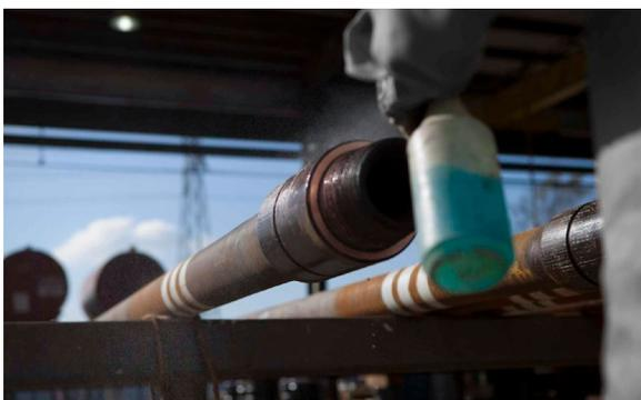
After completion of the inspection and repair operation, a rust preventative is applied to all connections on tools that are to be stored before the next use (Fig. 102). On tools that are to be used immediately, an API thread compound is applied to the threads and shoulders (Fig. 103).
