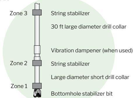
**Note:** In very mild crooked hole country the vibration dampener may be run in place of the short drill collar.
