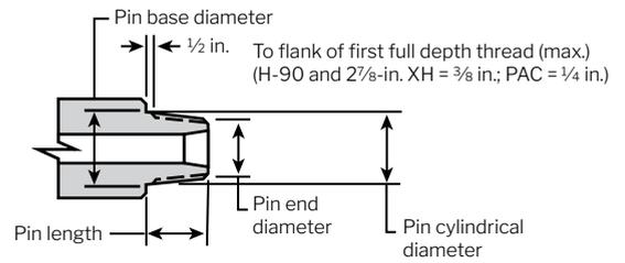
**Dimensional Identification of Pin Connections**
