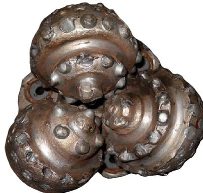
The bit in Figure 27 shows a broken medium, soft to medium formation roller cone bit that has been run off center. Note the cone shell, between rows of cutting structure, has been grooved by the rings of the uncut bottomhole formation.
