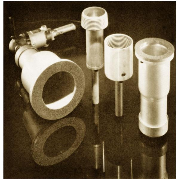
True alignment of the shoulder, perpendicular to the center line of the threads, is assured as the refacing tool mandrel is screwed on or into the connection threads (Fig. 98).
