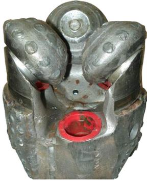
The bit in Figure 29 has suffered severe damage to the gauge and OD of the bit itself. The lugs have worn so badly that the shirttails are gone and some of the roller bearings are missing. The bit was run too long in an abrasive formation. When the bit is pulled like this, the last portion of the hole was drilled undergauge and the entire tapered portion of the hole must be reamed to the proper bit gauge.
