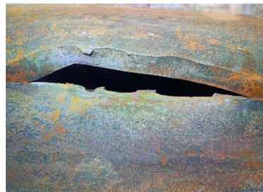
Large TFA Perforations from the Gator Perforator
