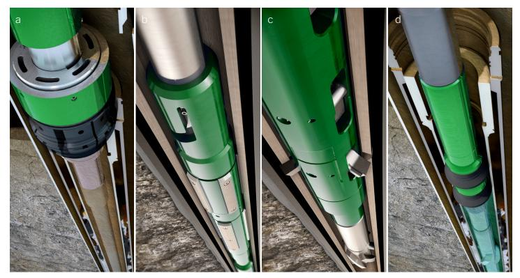
Prior to starting the cut, the wellhead seals are pulled (a) and the inline casing spear latches onto the casing (b). When the multicycle pipe cutter separates the casing string (c), high-pressure packoff seals the casing near the wellhead (d) to circulate out any cement, solids, and gas trapped in the annulus between the casing strings. Once the processes are complete, a trip out begins.
