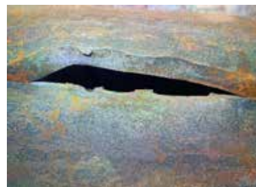
Large TFA Perforations from the Gator Perforator
