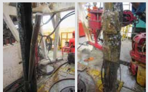
Figure 4: Recovered wireline tools previously lost in hole without any records.
