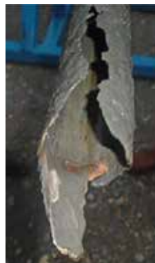
Figure 1: Heavily corroded 3½ in. production tubing.
