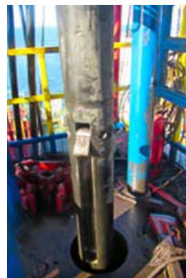
WIS hydraulic casing cutter tandem with 7 inch OD mud motor.
