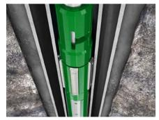
When the in-line casing spear is engaged, an overpull check is performed. Once a secure latch is established, the casing can be cut in tension to enable a faster cut.
