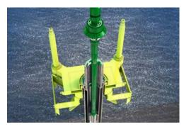
The casing is severed mechanically, and the wellhead spear remains engaged for a simultaneous retrieval of the casing section and wellhead.
