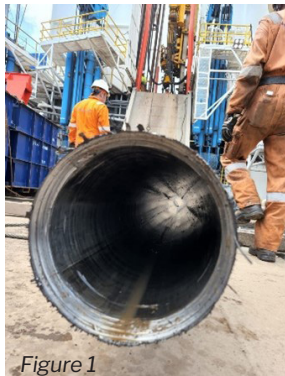
Figure 1: Cut 9 5 / 8 inch Casing 53.5ppf
