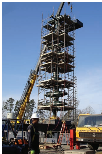
One of Thomas Tools' tallest snubbing stacks is shown—a rig-up of 21 \frac{1}{4} in BOPs.
