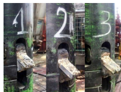
Figure 2: Post-run dull condition of pipe cutter knives
