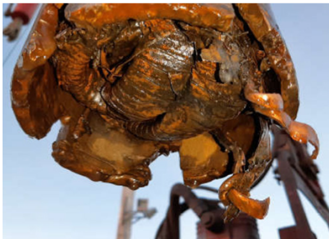
A customized Junk Basket with spring tines effectively recovers the ESP cable.
