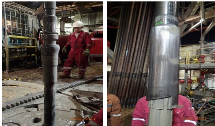
The recovered fish pulled up through the rotary table.
