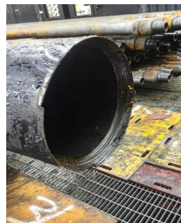
Casing cut in tension
