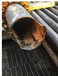
The ProMAXX-Hydraulic Spear passed through the damaged stump successfully
