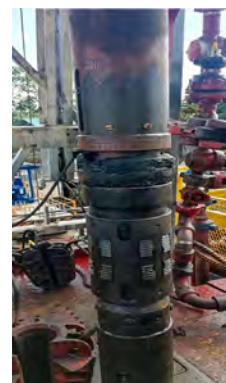
Figure 4: Successful recovery of lower Quantum Packer.
