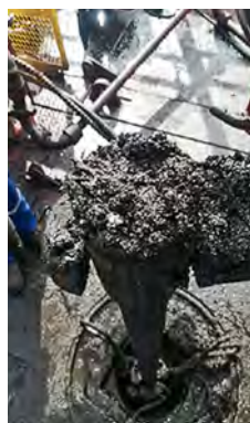
Figure 2: Debris inside the recovered upper Quantum Packer.
