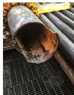
The ERS passed through the damaged stump successfully
