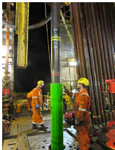
9 5 / 8 inch high-pressure casing patch hanging in the derrick ready to run in hole and install.
