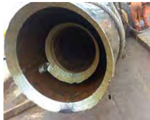
The 20 inch x 35 inch Cut Casings
