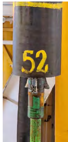
Wellhead and casing conductor retrieved with the ProLATCH System
