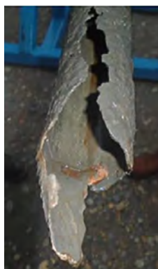
Figure 1: Heavily corroded 3 ½ in. production tubing.
