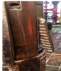
Figure 1: Post-run section mill (Note TruEdge cutting structure minimal wear)
