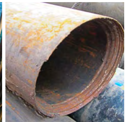
Casing cut successfully after a few minutes.
