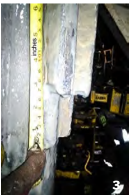
Photos 1-3 show the mill wear after the pilot milling run.
