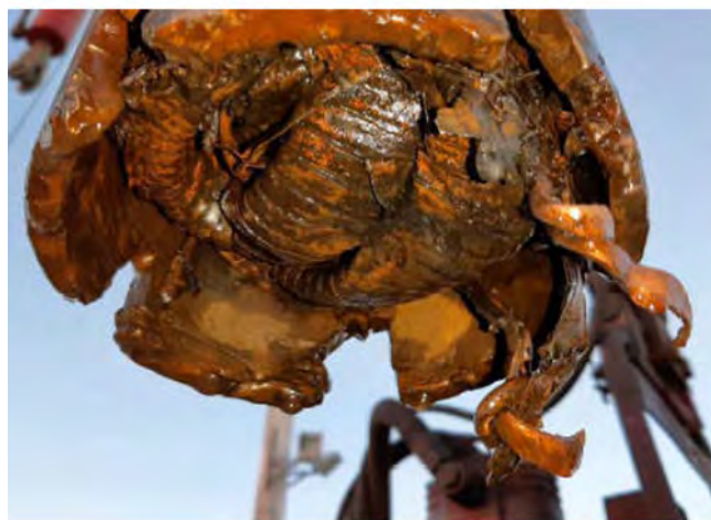
A customized Junk Basket with spring tines effectively recovers the ESP cable.
