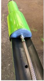
The 7 inch TrackMaster OH system with hydraulic anchor was oriented to the desired direction using MWD and properly set at 14,100 ft MD. After activating the hydraulic anchor, the shear sub was released from the whipstock
