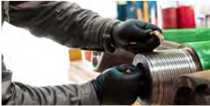
Tubular connection repair services include providing API stress-relief groove pins and bore back boxes, cold rolling thread roots, and phosphate coating to help prevent galling.
