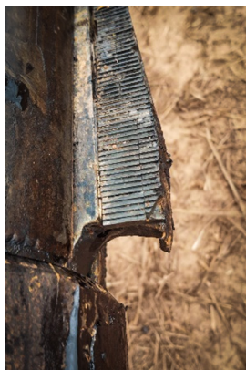
Left: K-Mill 5500 Section Mill knives calibration 8.5 inch OD Center: K-Mill 5500 Section Mill knives wear (hook shape) Right: Swarf recovered in string magnet
