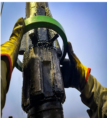
Left: K-Mill 5500 Section Mill knives calibration 8.5 inch OD Center: K-Mill 5500 Section Mill knives wear (hook shape) Right: Swarf recovered in string magnet
