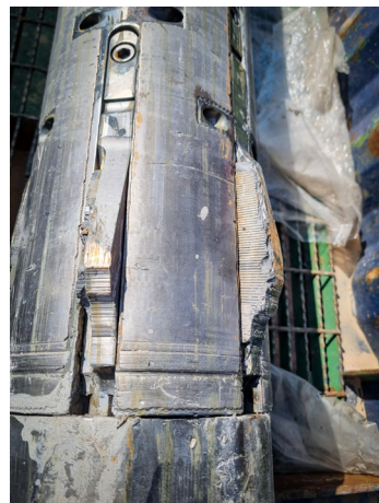
First and second run tools remained in good condition after successfully completing the section milling.
