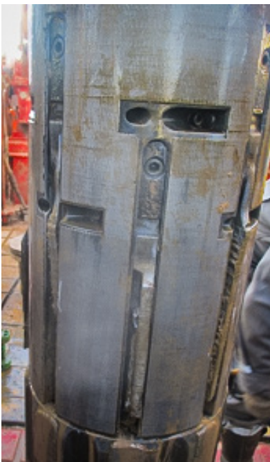
K-Mill tool, and TruEdge inserts after POOH during milling operation.
