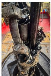
The successful recovery was confirmed by observing 6,000 lbs of additional weight while pulling out of hole, resulting in 100% of fish retrieval in surface.
